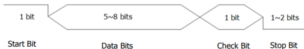
Figure 8.13 Schematic Diagram of UART Protocol
