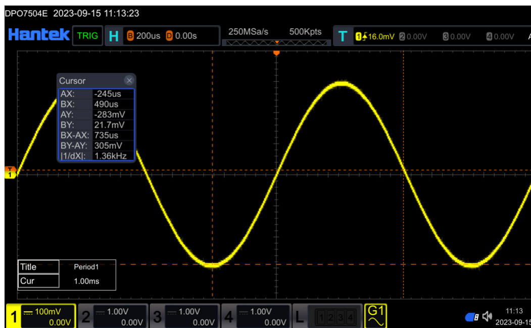
Figure 10.4 Track Measurement (after Horizontal Expansion)
